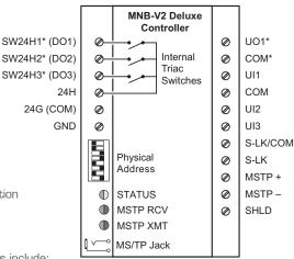
Asterisks indicate terminals that apply to the MNB-V2 controller but not to the MNB-V1.
